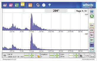
With the Twin Scope feature the acoustic noise impacts of the watch are displayed graphically. Displaying the Tic and Tac takes place simultaneously on the screen. The display is updated continuously after each nine half oscillation. This allows a detailed analysis of the beat noise and the state of the escapement system.
